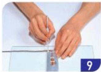
9 Soldering and locking cables
