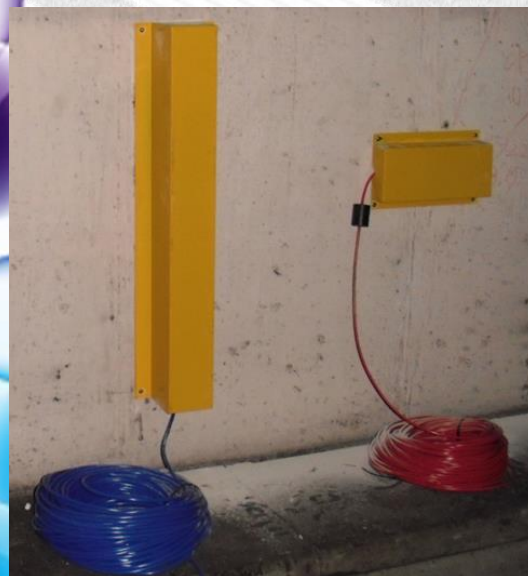
Installation Picture of EL Beam Inclinator with Cover
