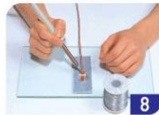
8 Soldering leading-wires of strain gage to the application
