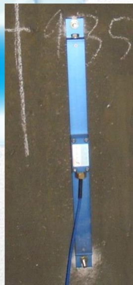
Installation Picture of EL Beam Inclinator
