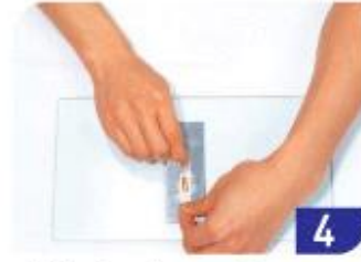
4 Aligning the strain gage
