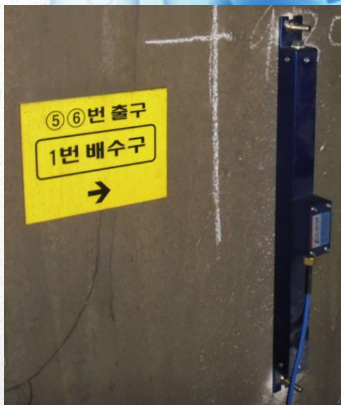
Installation Picture of EL Beam Inclinator
