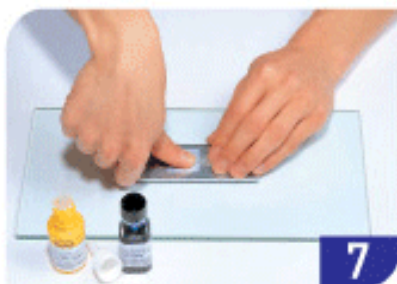
7 Pressing the strain gage
