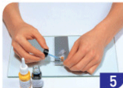
5 Applying the catalyst
