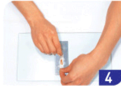
4 Aligning the strain gage
