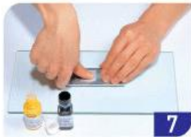
7 Pressing the strain gage
