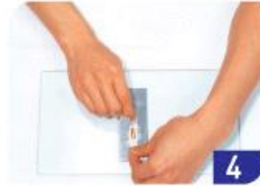
4 Aligning the strain gage
