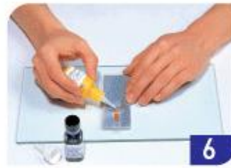
6 Dropping the adhesive
