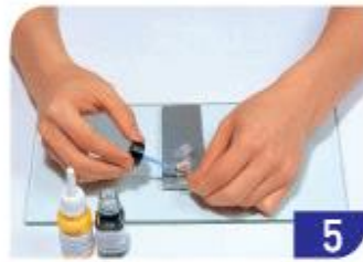
5 Applying the catalyst
