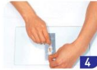
4 Aligning the strain gage
