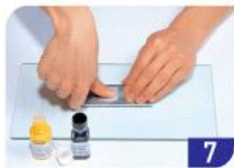
7 Pressing the strain gage
