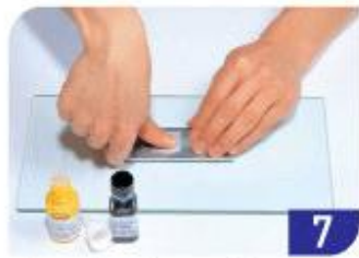
7 Pressing the strain gage
