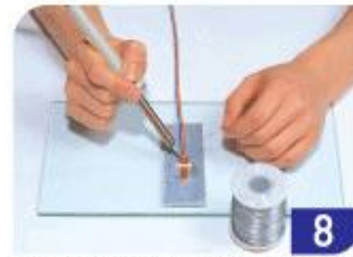
8 Soldering leading-wires of strain gage to the application
