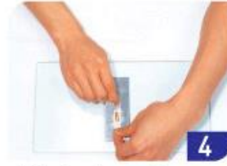
4 Aligning the strain gage
