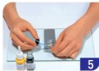
5 Applying the catalyst
